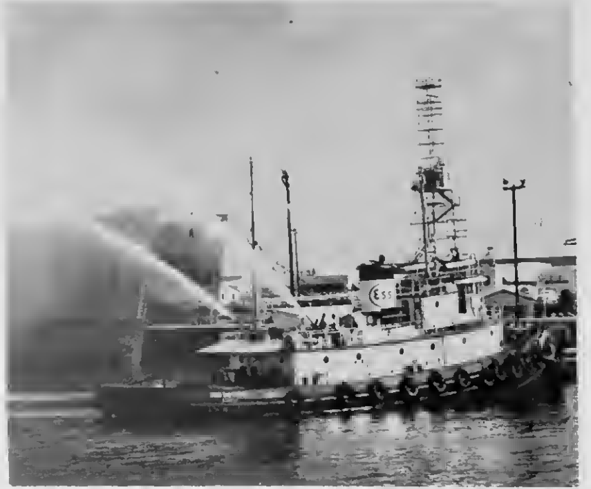
LAGO'S TUG Esso San Nicolas displays its water power during a fire drill in the harbor. Being extremely mobile, the tug can move about the scene of the fire and go to where it is most needed.
